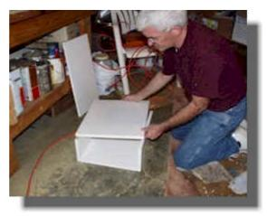
**Step 3.** Follow the instructions on the drawer slides as to separating the pieces for mounting. Mount the rails to the bottom of the Trash Box being careful to space them the same distance apart as the rails mounted on the cabinet bottom. Push rails together per the instructions and test for smooth operation.
